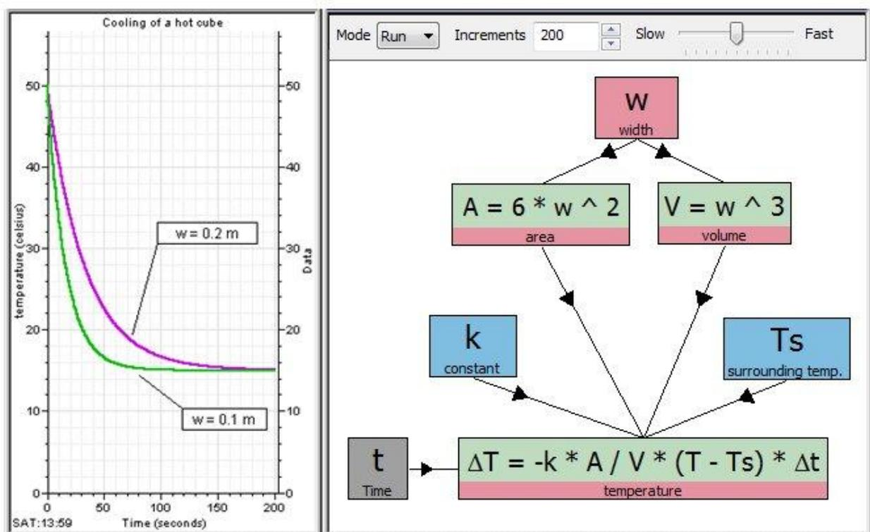
Fig. 6. Model and results for a cooling cube.
