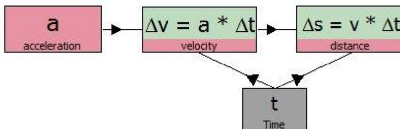
Fig. 4. Model for the motion of a falling object.
