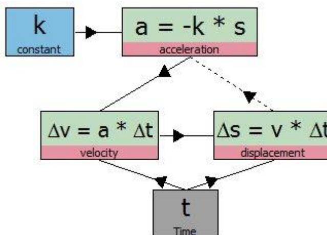
Fig. 5. Model for Simple Harmonic Motion.
